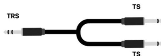
(TRS to double-ended TS adapter cable)
