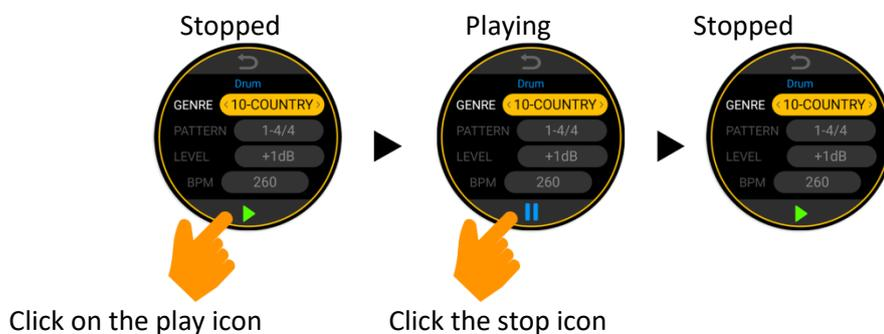
**Note:** With the DRUM menu open, single steps on the right footswitch will also perform the play/stop action for the Drum Machine.
