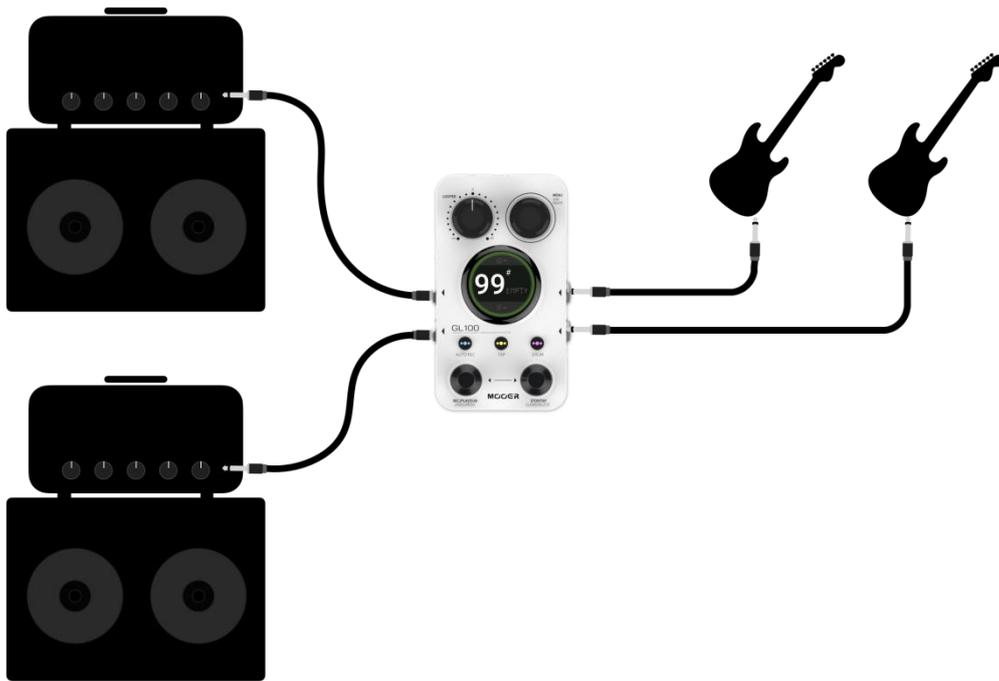
**Note:** For stereo / dual channel connection scenarios, you need to make sure that the "Input Setting" option in the MENU is set to "Stereo". See chapter [Input Setting](#).
