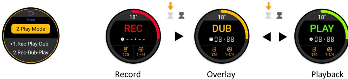
The "Rec - Dub - Play" mode makes it easier to start the second layer of overlay recording directly after finishing the first layer, without having to wait for the playback loop.
