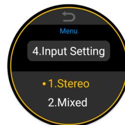
**Stereo:** Use this setting if stereo devices are connected at the inputs (which require a distinction between the left and right channel), such as stereo audio devices, some keyboards, stereo effects or two separate instruments.
