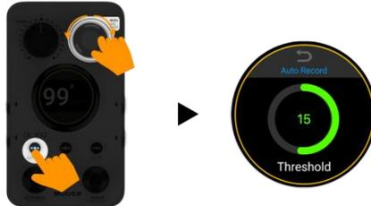
**Method 2:** Press and hold AUTO REC and simultaneously rotate the MENU knob to quickly adjust the threshold. The screen will automatically return to the previous view.
