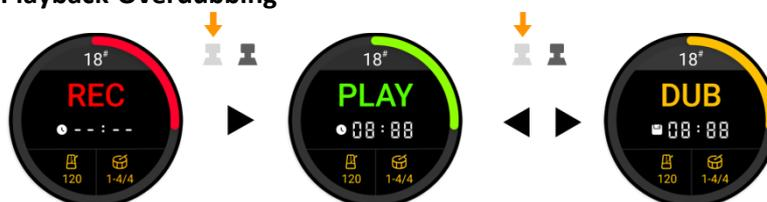
In this mode, you press the left footswitch to start Playback after recording the first layer of the loop and then press it again to start overdubbing the next layer.
