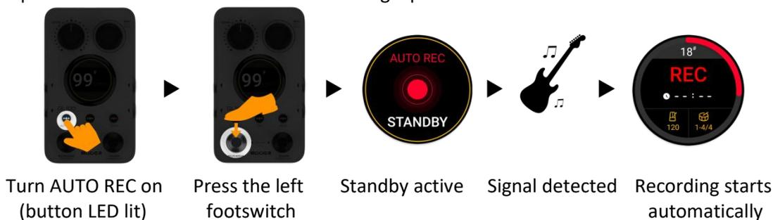
If you want to cancel the recording in standby mode, step on the left footswitch again, or press the AUTO REC button again to turn off the function.
