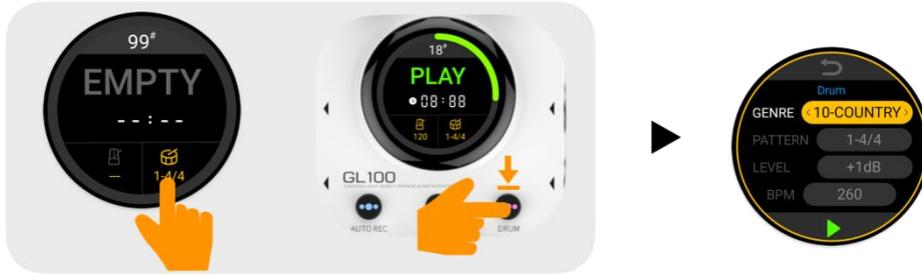
Click the **drum icon** in the LOOPER interface or long press the DRUM button on the panel to open the Drum Machine menu.
