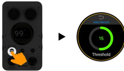
**Method 1:** Long press AUTO REC to enter the threshold adjustment menu, and adjust the threshold by rotating the MENU knob. Click the "back" symbol at the top of the screen to return to the previous view.
