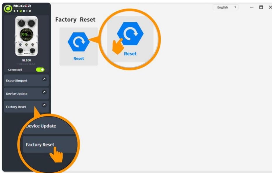
This operation has the same effect as using the "RESET" menu item on the GL100. After resetting, all user data in the unit is cleared and restored to factory state, including recorded and imported audio files, drum machine settings and menu setting items.
