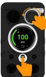
**Method 2:** Press and hold the TAP button and rotate the MENU to adjust the tempo.
