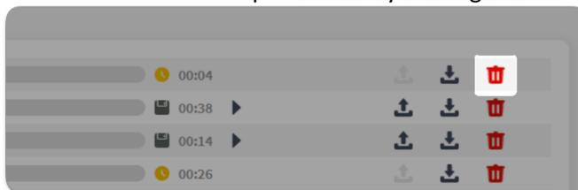
You can also delete individually or in batches by checking several target positions and then click **DELETE**.
