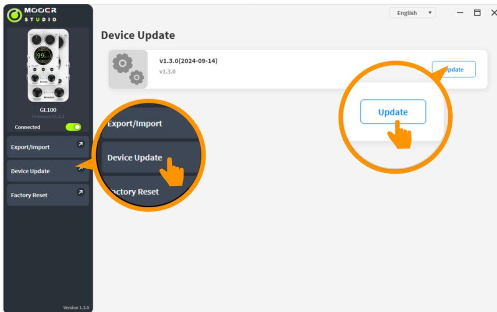
After clicking "Update", the device will reboot into update mode, and will automatically re-start into usage mode after displaying "Update Successful".
