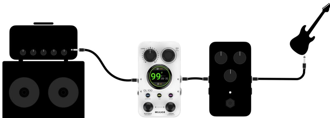
**Note:** In a single input scenario, if you want to avoid a situation where only one output (or one side of the headphone) gets the pass-through signal from the input, open the MENU screen and change "Input Setting" to "Mixed". See chapter *Input Setting*.
