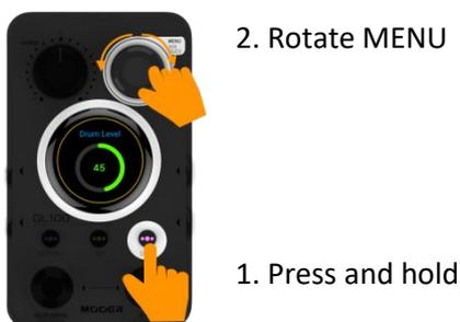
**Note:** For quick and easy adjustment of the balance between the individual volumes, Drum Machine volume and Looper volume are **global parameters** and are not saved with the storage location.
