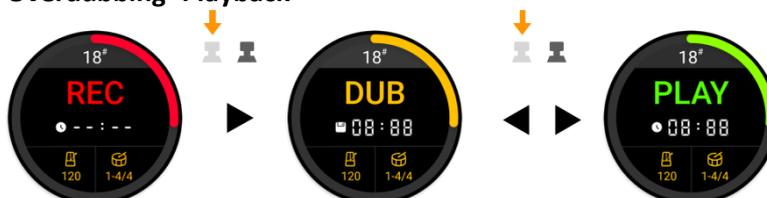
This mode can be used to record the second layer of the track immediately after finishing the first layer by pressing the left footswitch. The first layer will be played automatically while you overdub the second layer.
