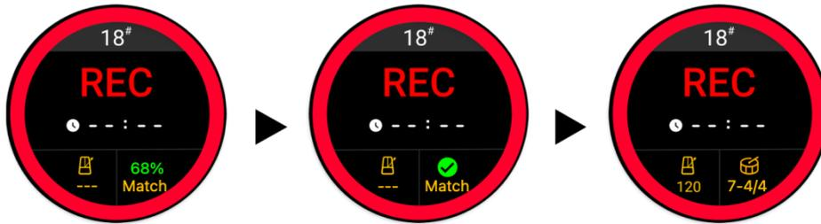
The matching process lasts for about 8 seconds. It should be noted that the recording of the phrase does not have to end after the Drum Machine produces the result. You can continue to play, but everything you play after the matching is completed will not be used for the matching process.
