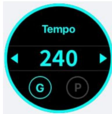
**Preset Mode:** Tap the screen to select P (Preset Mode), then press the footswitch twice in quick succession. M2 will set the Tempo speed based on the time interval between the last two footswitch presses, applying it to the modulation effect speed and delay effect time of the current preset sound. You can also adjust the Tempo speed by tapping the arrow icon on the screen.
