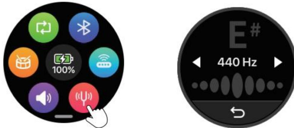
**Exit Tuner:** Tap the back arrow icon or press either footswitch to exit the tuner.
