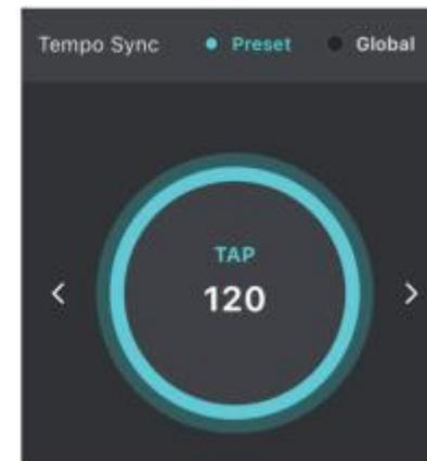
Click the icon to enter Tempo speed settings. You can choose the mode for Tempo Tap Tempo, either synchronizing the speed of preset effects (modulation and delay) or globally (preset effects and drum machine). You can set the speed by continuously tapping the circle area or use the left and right arrows for precise adjustments.
