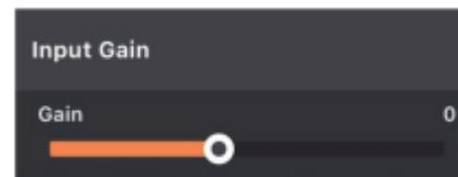
You can adjust the gain according to the instrument or preamplifier connected to the M2 to ensure that the input signal operates within a normal range.
