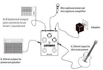
Please turn On the LINE IN switch when using the external micro phone amplifier
