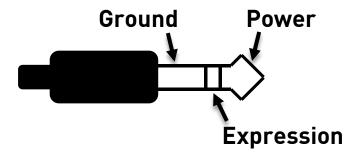
Expression pedals with TS (Tip Sleeve) plugs will not work correctly with the Aftershock.
