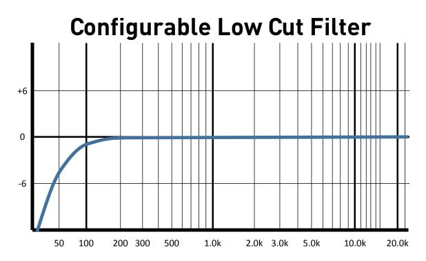
The Parametric EQ and the Low Cut filter are configurable using the Neuro App. By default, the parametric EQ is disabled (flat), and the Low Cut filter is set to 10 Hz.
