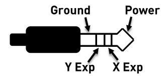
Third party passive expression pedals can be used as well, as long as they have a TRS (Tip Ring Sleeve) plug with power on the tip, expression (the wiper of the potentiometer) on the ring, and ground on the sleeve, as seen in the diagram below.
