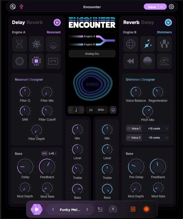
The Encounter's Sound editor contains mixing and EQ controls in the center along with internal channel routing options. On either side are parameters for both the delay and reverb engines, ranging from classic delay and reverb controls (*Base*) to flexible, engine-specific parameters (*Designer*).
