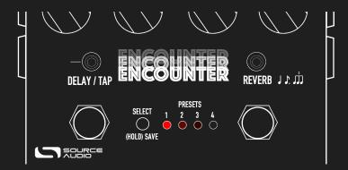
Encounter has 128 preset slots. User Presets store all editable parameters. This includes the knob positions, parameter settings, routing options, external control, and the full list of Neuro/MIDI accessible parameters. After a preset is recalled, you can always tweak the top-level controls in a performance situation by turning the knob. The knob parameter will then "jump" to the current knob position as it is rotated.
