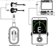
Pair the Transmitter and Receiver by making sure that they are set to the same wireless channel. The AS8 Transmitter has six channels; use the channel select button to change the channel as needed.
