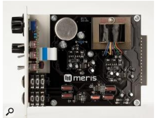
The circuitry, based on the venerable API 312, uses modern surface-mount components and employs Cinemag input and output transformers.
