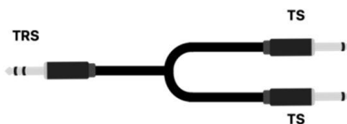
(TRS to dual TS adapter cable, Y-format cable)
