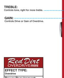
Power Requirement: 9VDC Center Negative Power Supply Required
